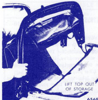
Fig. 6 - Lifting Top Out of Storage
